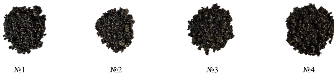
Fig. 3. Samples of solid metal sulfates obtained by drying
