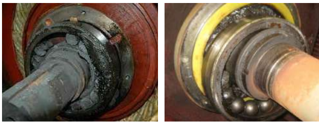
9-rasm. Elektr motor rotorining podshipniklarining shkastlangan qismining ko'rinishi
