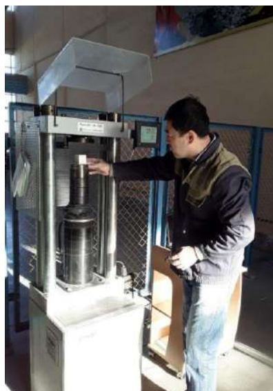
3-rasm. IP-1A-1000 PK modeldagi gidravlik sinov mashinasida tajriba o'tkazish jarayoni (Braziliya usulida)
